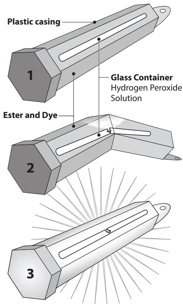
1. The glow stick is filled with a chemical compound called an ester and dye. Inside, a small glass container is filled with hydrogen peroxide.
