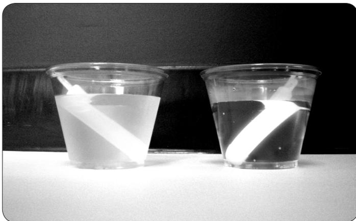
The glow stick in the hot water (right) glows brighter than the glow stick in the cold water (left) because the higher temperature increases the speed of the chemical reaction.
